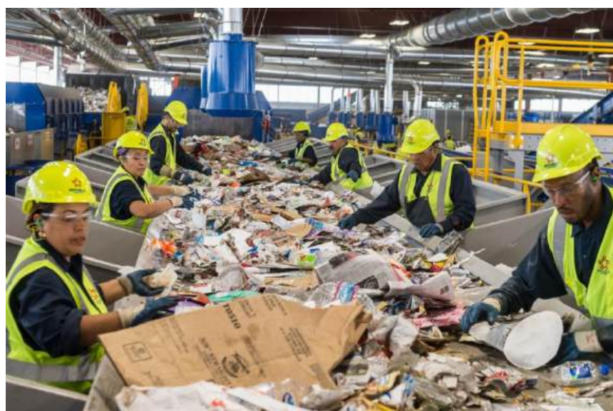
Figure 3.3: Impression of a part of the Industrial Recycling Hub (handpicking station)
