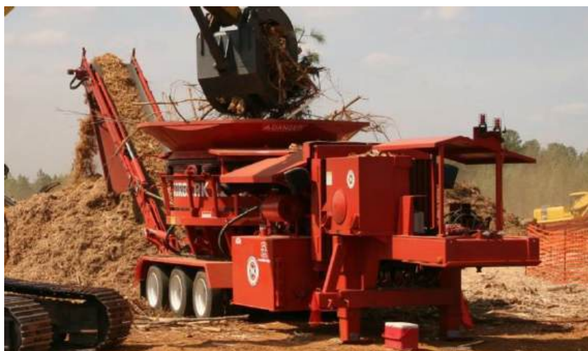
Figure 3.4: Shredding by means of a tub grinder
